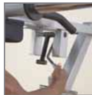
The spring loaded lockout handle is within easy reach at all times.
